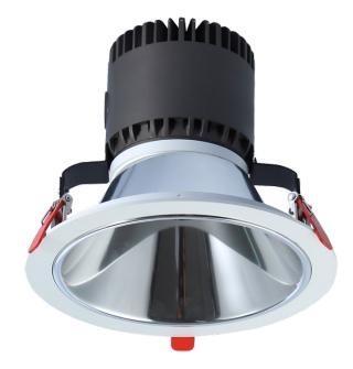
The Risa LED is a 144mm diameter downlight which uses a CREE LED engine. The heatsink is constructed from diecast aluminium complete with aluminium bezel and reflector. The bezel features a 40mm recess detail creating a glare friendly cut-off which is also an aesthetically pleasing architectural detail.
