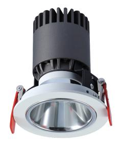
The Risa Mini LED is a 96mm diameter downlight which uses a CREE LED engine. The heatsink is constructed from die-cast aluminium complete with aluminium bezel and reflector. The bezel features a 40mm recess detail creating a glare friendly cut-off which is also an aesthetically pleasing architectural detail. The Risa Mini is available with a 1,100 lm output with 15°, 24°, 30°, 36°, and 45° beam angle options.
