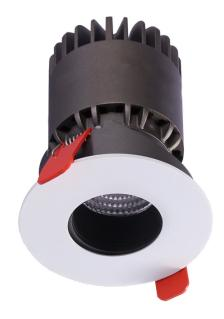
The Risa Pin Adjustable LED is a 90mm diameter adjustable downlight which uses a CREE LED engine. The heatsink is constructed from die-cast aluminium complete with aluminium bezel and reflector. The bezel features a 38mm aperture detail creating a pin-like appearance with a sharp beam angle.
